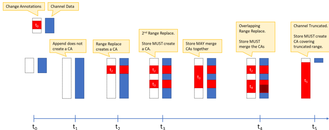
Figure 20: Example showing how change annotations (CA) work over time for channels. Blue box = channel data, white box with red label = change annotation. The size of the white box is intended to show that the annotation is for the entire corresponding channel (blue box).
