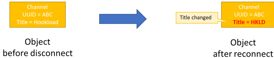
Figure 41: Example of update to data object. While disconnected, the channel's title has been changed (from "Hookload" to "HKLD").
